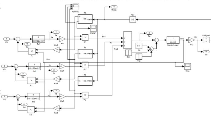
Fig. 12 Simulink model of BLDC Motor
