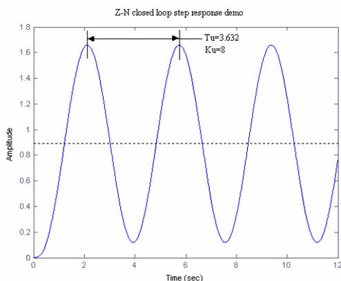
Fig.6 Z-N closed loop parameter evaluation for sample system
