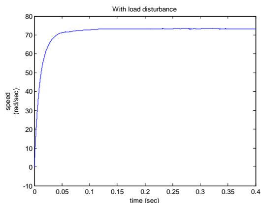
Fig. 19 Speed response of the drive with load disturbance
