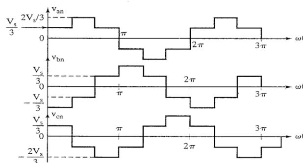
Fig.4 Three phase output voltages on a three-phase VSI in 180° mode
