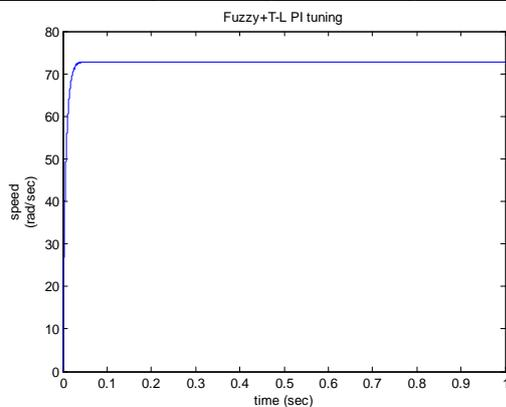
Fig. 16 The speed response with Fuzzy PI Controller
