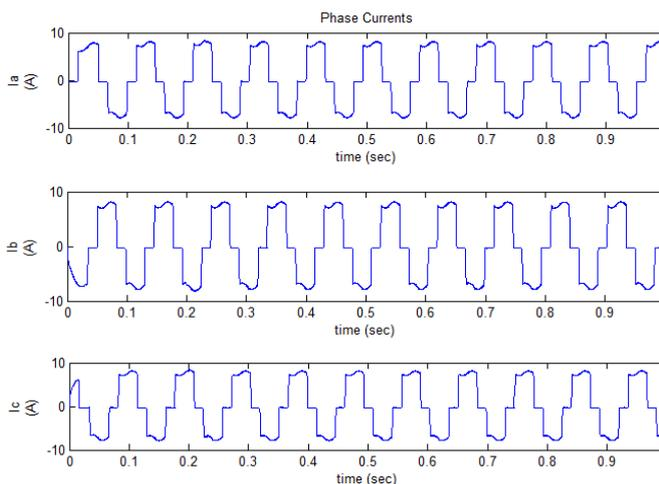
Fig.22 Three phase currents of the BLDC motor
