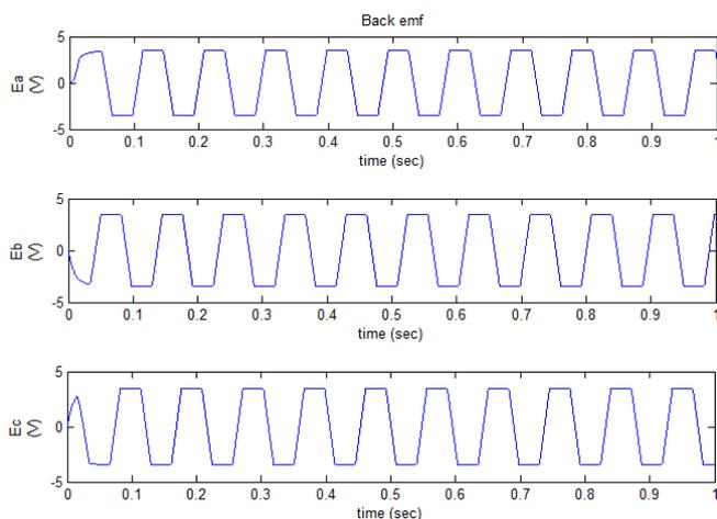
Fig.21 3-Φ Trapezoidal Back emf Waveform of the BLDC motor
