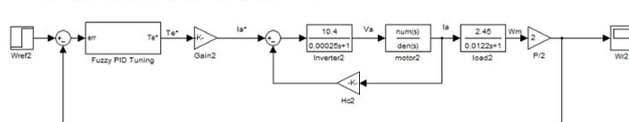
Fig. 14 Closed loop Transfer function of the BLDC Motor Drive
