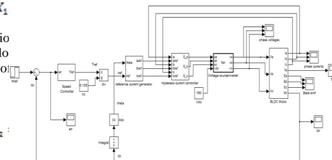
Fig. 13 Overall Closed loop model of the drive
