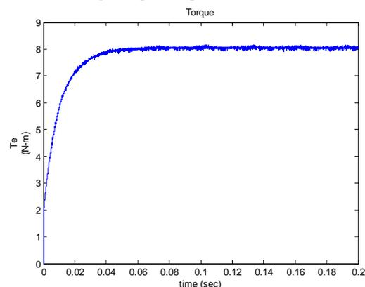
Fig.18 Electromagnetic torque developed in the drive
