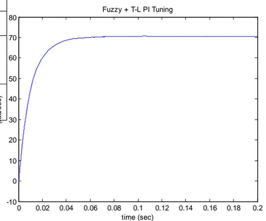
Fig. 17 Speed response of the Drive
