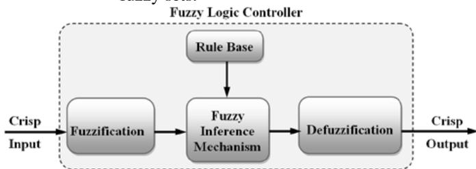
Fig.8 The structure of a fuzzy logic controller
