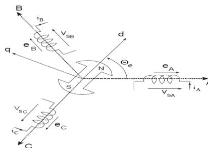
Fig.2 Position of the rotor with respect to the phase A
