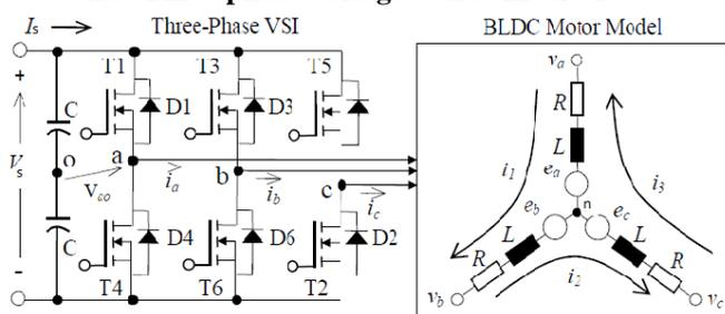
Fig.3 Configuration of BLDC motor and Three Phase VSI system
