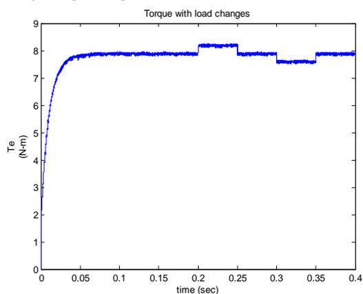
Fig.20 Torque developed in the drive with load disturbance
